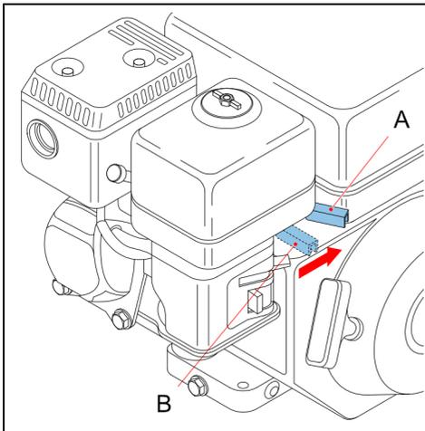
1. Completely push the throttle lever (A) into the [LOW/MIN]-position (B).
