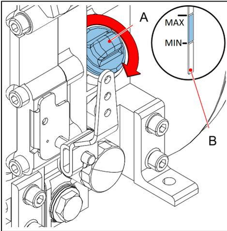
5. Add new engine oil to the correct level via the opening of the oil tank filler cap (A).
