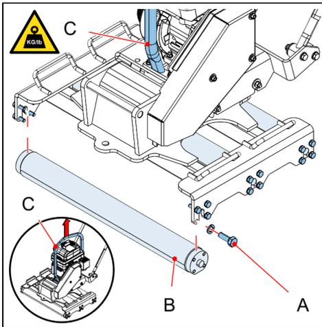
1. Raise or tilt the machine with the lifting frame (C) until there is enough clearance to access the applicable roller (B).
