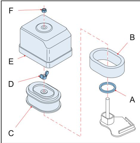
1. Remove the nut (F) on top of the air filter housing (E).
