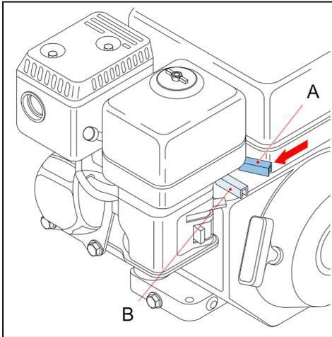
3. Completely push the throttle lever (A) into the [LOW/MIN]-position (B).
