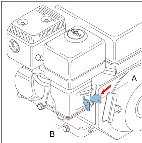
3. Push the fuel tap (A) into the closed (B) position.
