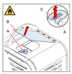
**1.** If applicable: lift the rubber cover (B) on top of the fuel tank (A).
