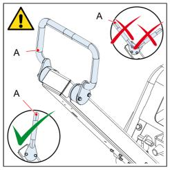
1. Push the directional handle (A) into the [MID/Stationary]-position.
