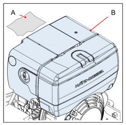
**12.** Clean the exposed surface of the engine (B) with a clean, soft, absorbent cloth.
